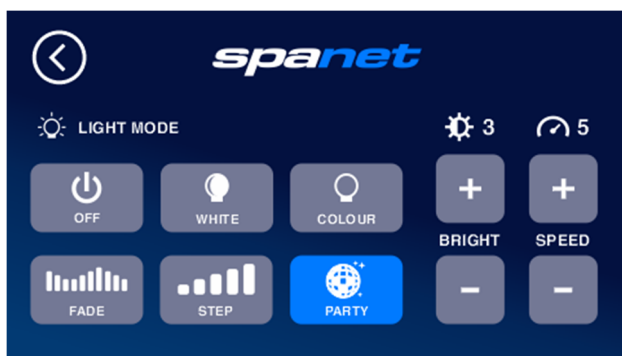
Party Effect Dsico flashing transition through all colours Light effect transition speed (RH slider) Light brightness adjustment (LH slider)
